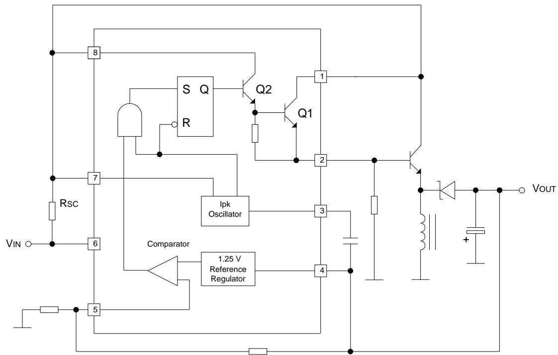
Voltage Inverting With External PNP Saturated Switch
