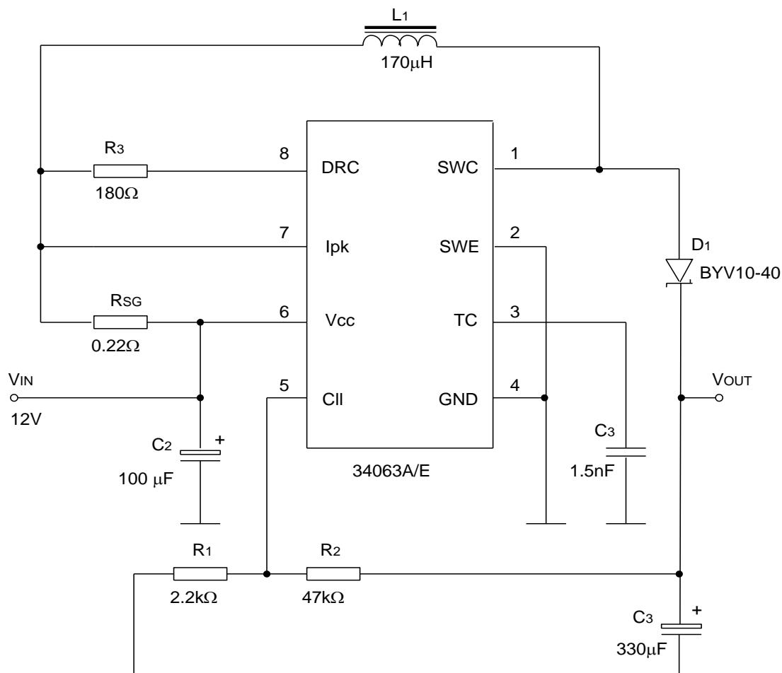
Test Condition ( $V_{OUT} = 28$  V)
