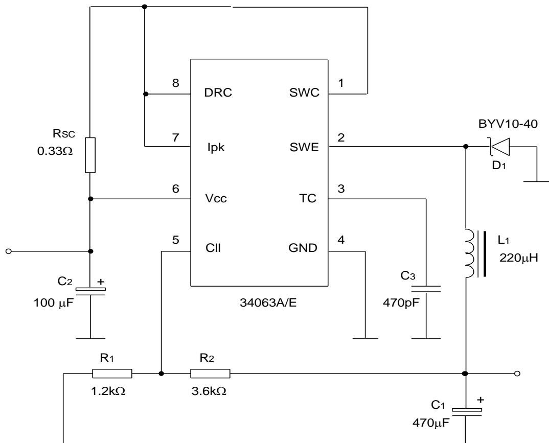
Test Condition ( $V_{OUT} = 5$  V)
