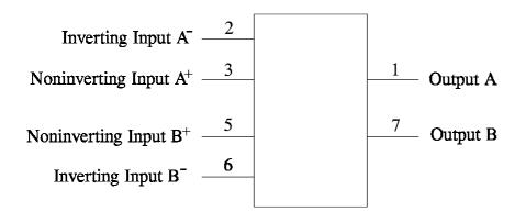
Pin 4 = Supply Voltage  $V_{-}$ Pin 8 = Supply Voltage  $V^{+}$
