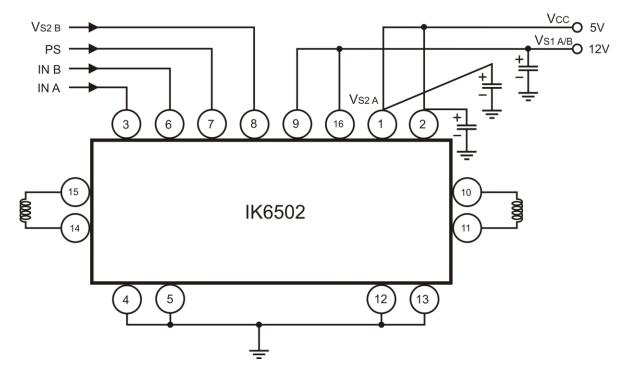
Note 1: Connect the  $V_{S2A}$  terminal to the lower supply voltage (5 V).
