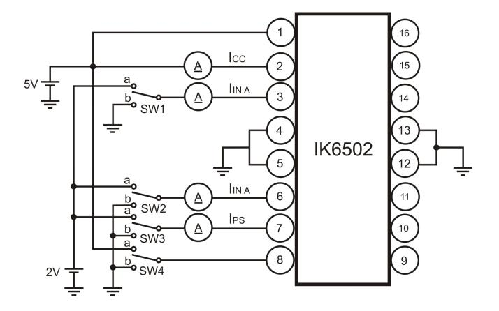
Test Circuit 1.  $I_{CC1}$ ,  $I_{CC2}$ ,  $I_{CC3}$ ,  $I_{IN A}$ ,  $I_{IN B}$ , and  $I_{PS}$
